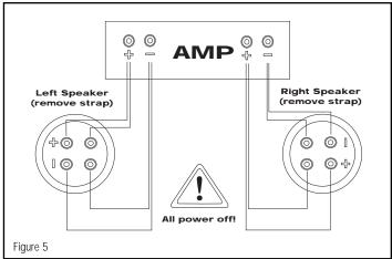
one cable to the tweeter binding posts and another to the woofer binding posts. Run both
